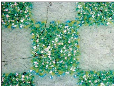
Image: Checkerboard print by a Canon MP620 printer on instant dry photo gloss inkjet paper
